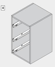
Fasten runners to cabinet sides with required screws into pre-bored holes. Add extra screws as required for strength.
