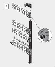
Determine runner locations and set templates on the bar by using the integrated scale.
