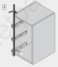
Bore Ø2.5mm pilot holes through templates for front and middle mounting positions.
