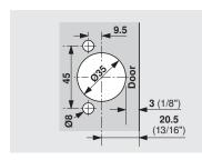
Cup centerpoint and MINIPRESS / MINIDRILL set-back position is **20.5** (13/16") for COMPACT hinges.
