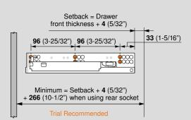
NOTE: To meet specified weight capacities, two screws in front and back are required.
