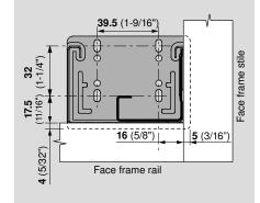
NOTE: For frame installation. Min. 3 screws per socket.
