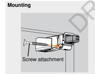
BLUMOTION for doors mounts anywhere on the hinge-side style of the cabinet using a 1-1/4" (or 2" screw when using spacer).
