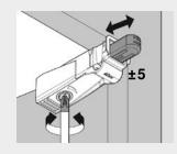
Use a Phillips or POZI screw driver to adjust the contact point in or out 5 mm. Adjust out for larger, heavier doors or in for smaller, lighter doors.
