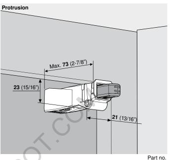
BLUMOTION mechanism 971A9700 #8 x 1-1/4" wood screw 8114Z
