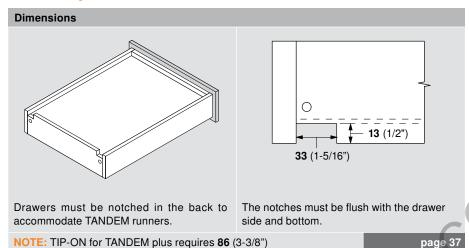
Make the back panel shorter and extend the drawer bottom to the back of the drawer.
