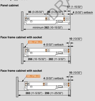
NOTE: To meet specified weight capacities, two screws in front and back are required.
