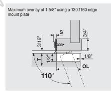
Hinge arm protrusion (S), and door protrusion (P), for edge mount mounting plates
