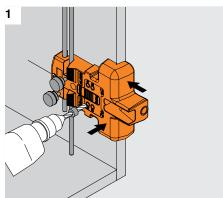
Position template on marking line and use a Ø2.5mm or Ø5mm drill bit to bore into cabinet side panel for various BLUMOTION adapter plates.
