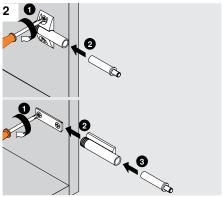
Depending on your mounting plate option, install adapter plate and insert BLUMOTION for doors.
