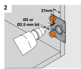
Bore holes for mounting plates with Ø5 or Ø2.5mm bit.
