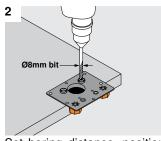
Set boring distance, position in hole and bore Ø8mm dowel holes.
